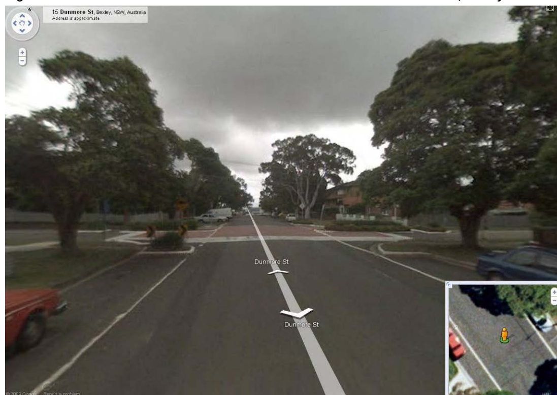
Figure 6: Raised Threshold at the intersection of Dunmore St & Monomeeth St, Bexley
